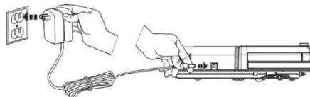
Turn off the vacuum cleaner on the main switch to prevent it from moving. Then connect the 230 V power adapter directly to the vacuum cleaner. A full battery charge will indicate that all LEDs on the top panel are on.
