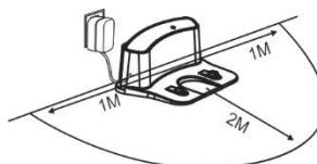
3. Place the vacuum cleaner in the charging station and battery will start charging automatically.
